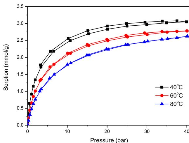
**Figure 9.**  $\text{CH}_4$  adsorption–desorption isotherms on pure carbon spheres (sample RF 700).
