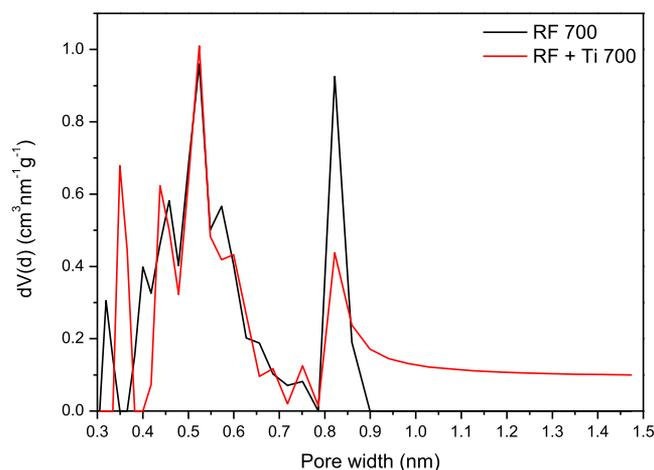
**Figure 8.** Pore size distribution of pure carbon and composite samples.
