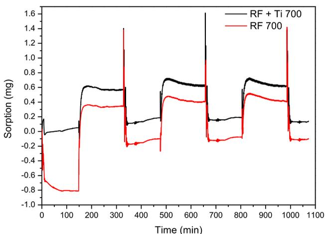
**Figure 11.** Thermogravimetric analysis curves for the CO<sub>2</sub> adsorption–desorption cycles.
