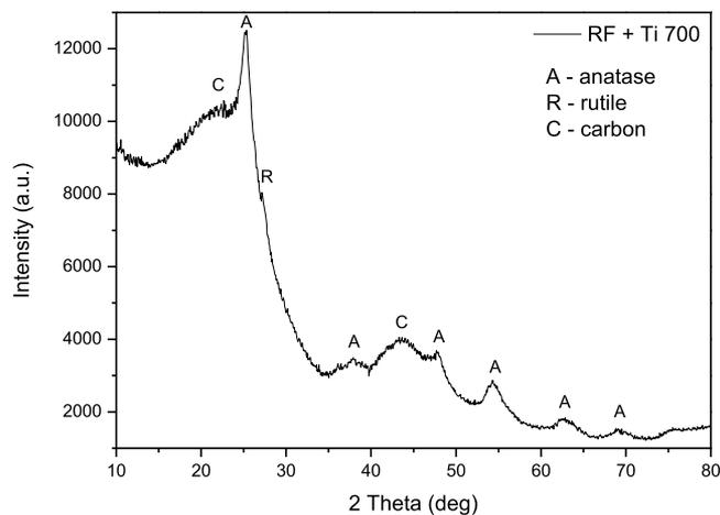
**Figure 5.** XRD diffractogram of the RF + Ti 700 sample.
