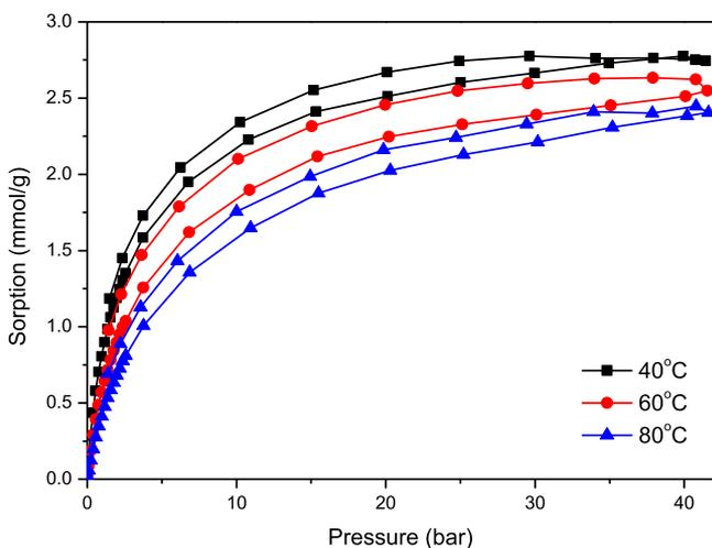
**Figure 10.** CH<sub>4</sub> adsorption–desorption isotherms on composite titania–carbon spheres.
