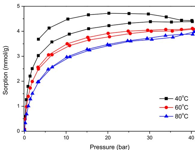
Figure 13. CO<sub>2</sub> adsorption–desorption isotherms on carbon spheres.
