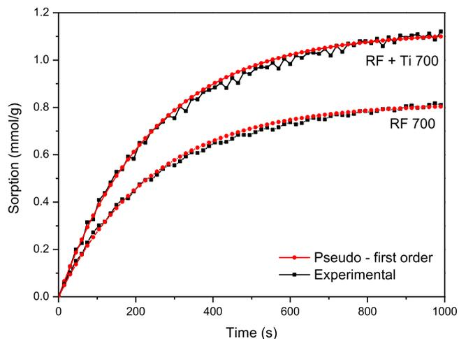
**Figure 12.** Experimental CO<sub>2</sub> uptake for the samples RF 700 and RF + Ti 700 and the corresponding fit to the kinetic model.
