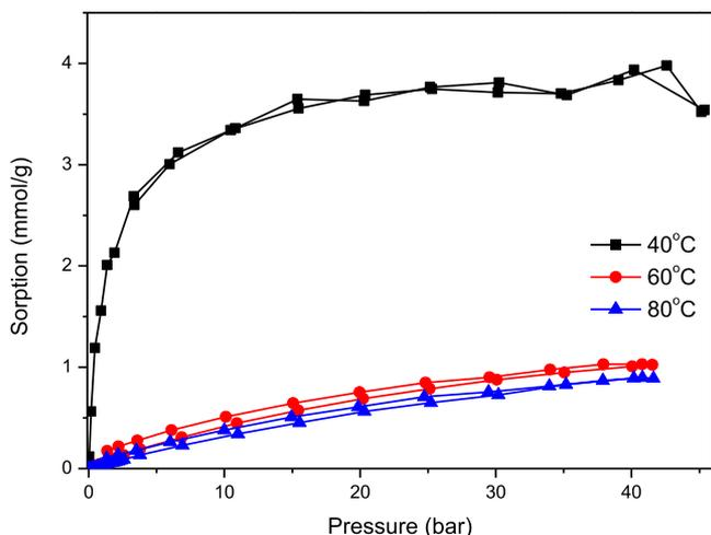
Figure 14. CO<sub>2</sub> adsorption–desorption isotherms on composite titania–carbon spheres.
